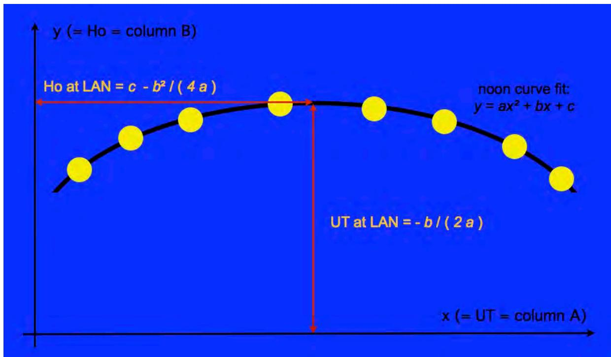
The noon sight in principle allows you to determine the position and indeed the latitude can be measured to a good accuracy. However, in practice the inferred longitude is often inaccurate due to the difficulty of marking the precise moment of LAN. The sun hangs at its maximum altitude for a couple of minutes and every four seconds of uncertainty in the time of LAN introduce an error of 1 arc minute of longitude.
