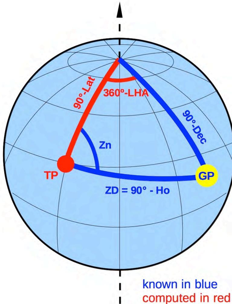
If both the azimuth ( $Z_n$ ) and the altitude ( $H_o$ ) of a celestial body is known, then it is possible to obtain a fix for the “true” position (TP) from observing that one body alone. The spreadsheet *one\_body\_fix.xls* solves the navigation triangle in this scenario. The GP is characterized by its declination (cell A2) and Greenwich Hour Angle (B2). The azimuth ( $Z_n$ ) is entered in cell C2, and the observed altitude ( $H_o$ ) goes into cell D2. The TP coordinates are displayed in row 6.
